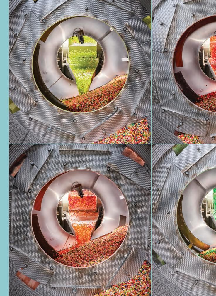
Assortments mix together in a tumbler, which also filters out misshapen treats, known as Belly Flops. Too-small morsels drop through holes in the first roller; perfect ones land on a conveyor below the second; and big'ns get stuck in the third.
