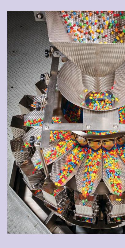
A machine funnels candies into 16 bags of equal weight. This machine can sort beans into bundles of up to 9.8 ounces, but Jelly Belly also sells its treats in bulk—up to 3 pounds, or 1,200 wee sugar bombs.
