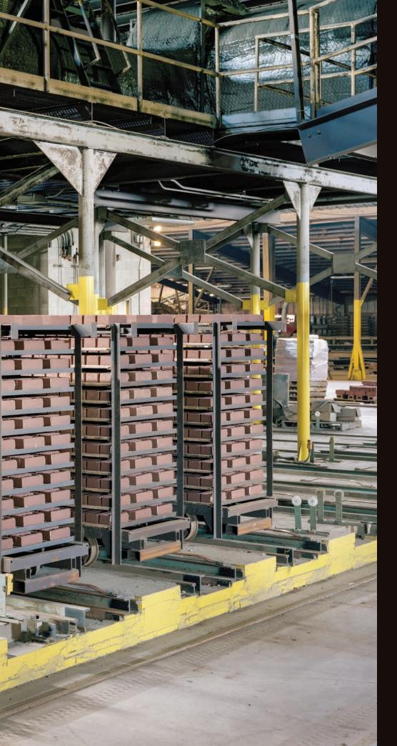
Workers remove the bricks from their molds and cure them for 36 hours in wheeled drying racks, which are set on tracks. The machinery may be over a century old, but the technology is highly automated, directing leftover heat from used kilns into this preliminary drying areas.
